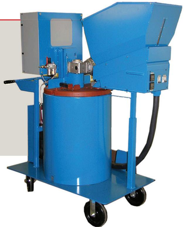
The wax level in the conditioner is monitored to ensure it is always properly filled and ready to feed your wax injector system:
